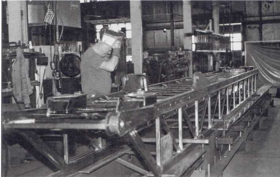
Inspecting a ladder that will be installed on a fire truck, to ensure its strength and stability.
